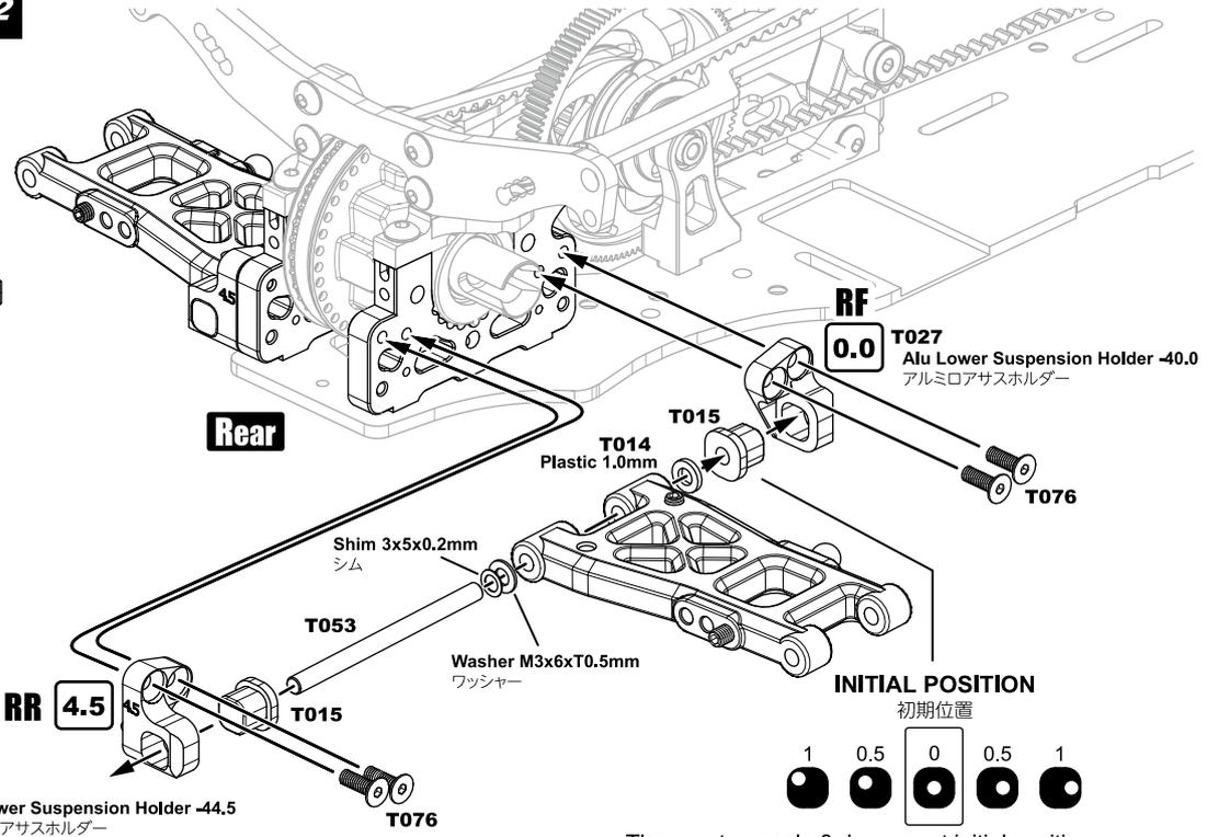
The rear toe angle 3 degrees at initial position.
