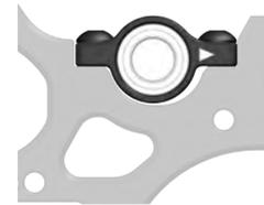
Wheelbase adjustment (forwards/backward  $\pm 1.0\text{mm}$ ) can be made by the orientation of the ride height adjuster.
